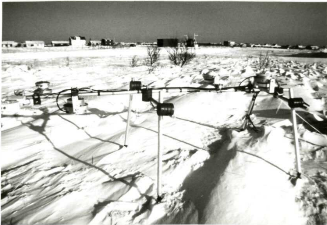
Figure 4.3: The automatic radiation station mounted at the airfield Andenes.
