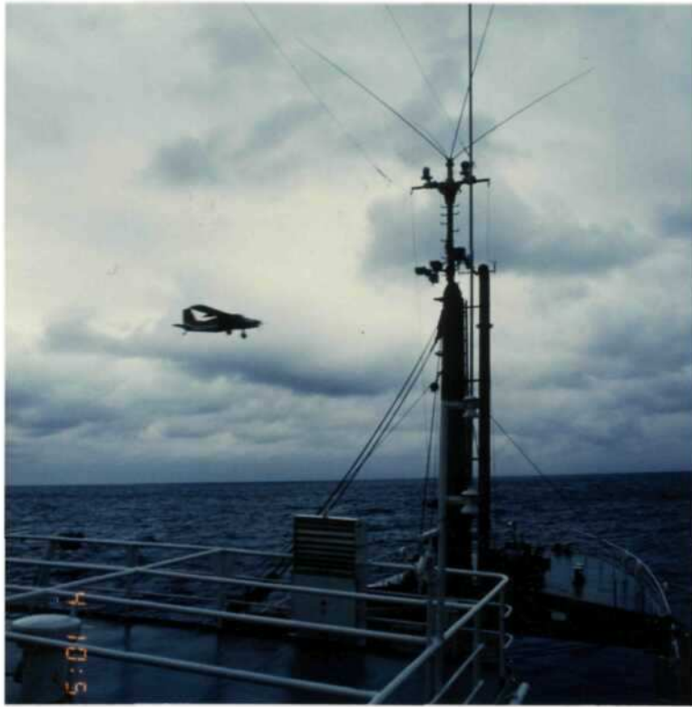
Figure 2.3c: Fore-deck station with aircraft DO-128 during a calibration flight.
