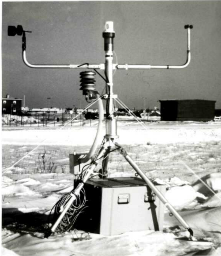
Figure 4.2: The automatic station for meteorological surface data mounted at the airfield Andenes.
