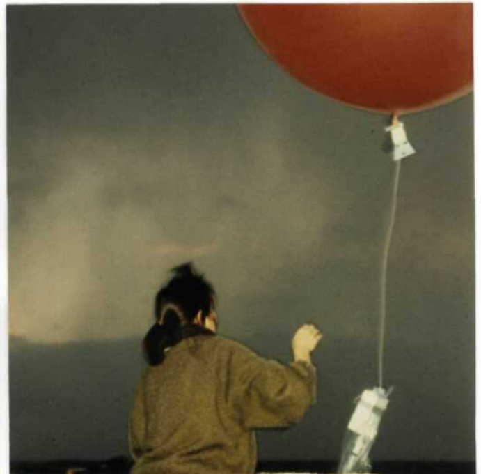
Figure 2.3a, b: Inflating and starting a balloon with radiosonde RS80/N15 by G. Fischer.
