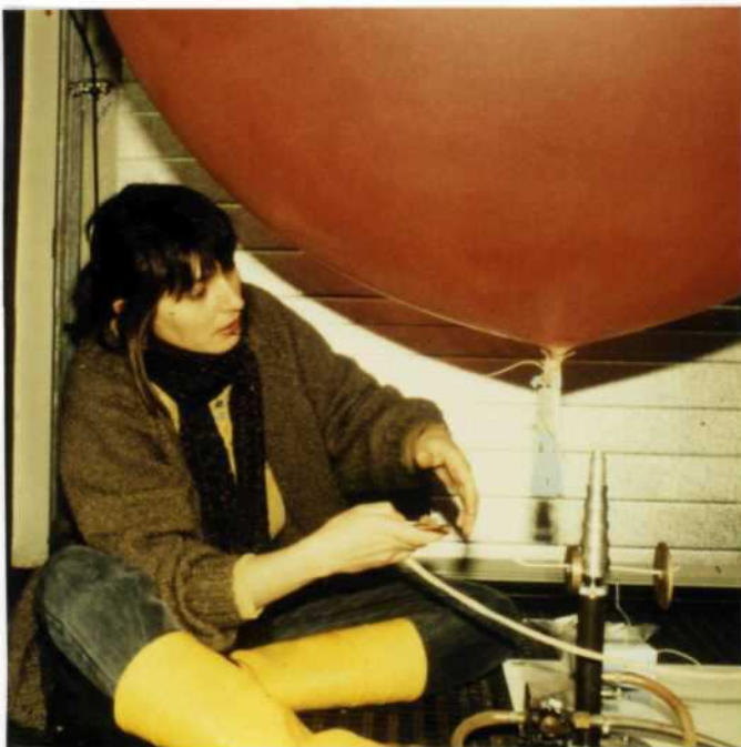
Figure 2.3a, b: Inflating and starting a balloon with radiosonde RS80/N15 by G. Fischer.
