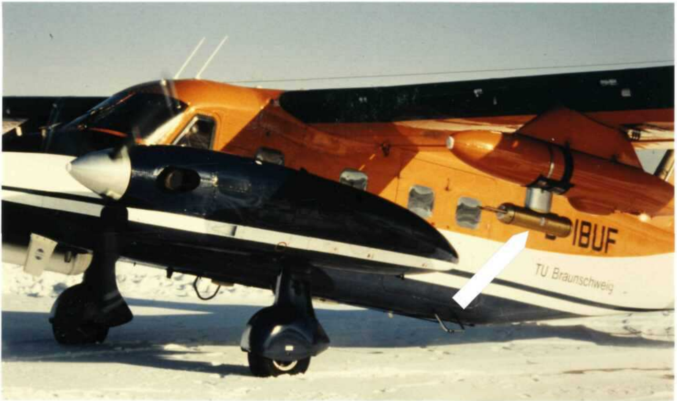
Figure 5.18: The research aircraft DO-128 of the Technische Universität Braunschweig showing the location of the 2-D-grey probe under the left wing.
